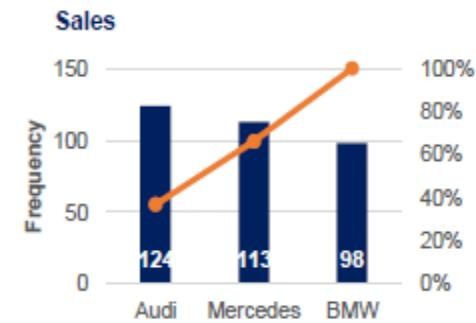
The Pareto diagram is a special type of bar chart where the categories are shown in descending order of frequency, and a separate curve shows the cumulative frequency.
